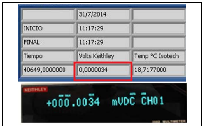
Fig. 6. Comparison between software configuration for measuring on channel no. 1 and measured data from equipment in channel no. 1.
